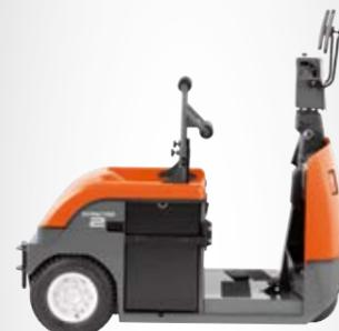
Compact stand-in towing tractors for horizontal transport, especially short distance with frequent on/off
