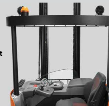
Duplex Tele Mast
